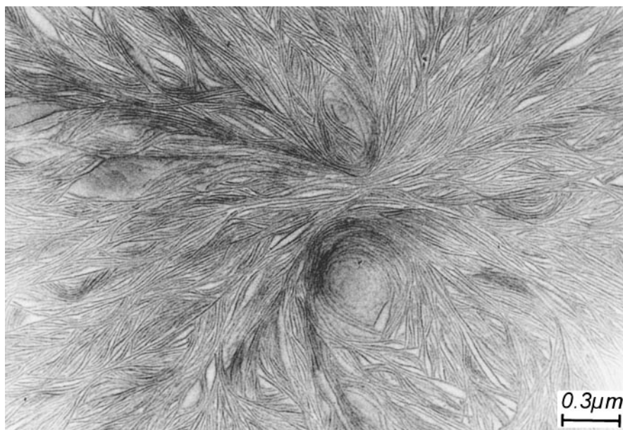
Figure 3 BF electron micrograph of an iPS sample as in Fig. 2, which was further treated at 190°C for 1 min and then quenched to room temperature.
